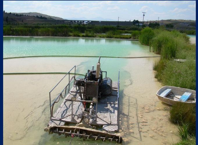
Figure 3. Pump barge and equipment
